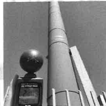
Radiation from 5G tower: .004 W/square meter
