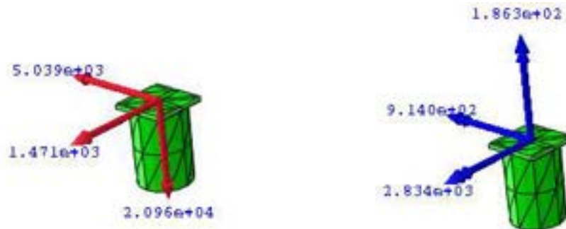
Figure 44. Force and Moment components for base of exterior Column 1A under seismic loading.
