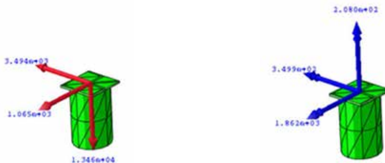
Figure 50. Force and Moment components for base of interior Column 1A under seismic loading.
