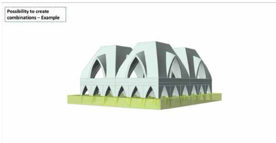
Figure 4. Possibility of clustering several structural units together to create larger houses. There can be different clustering possibilities beyond the one shown.
