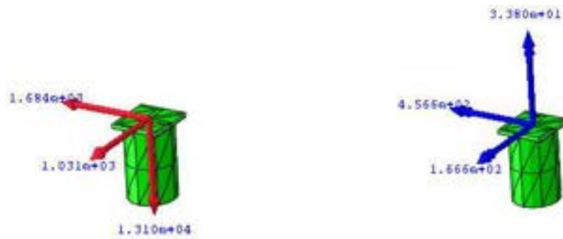
Figure 65. Forces and Moments in Column 1A for Wind Load case 3.
