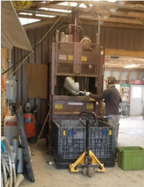
Figure 13: Recycle materials loaded by hand or shovel into baling chamber
