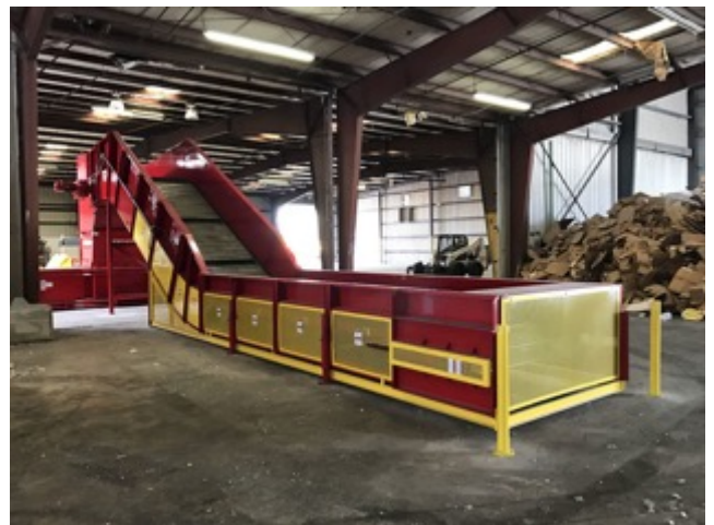
Figure 15: Recycle materials loaded onto above ground conveyor belt into hopper above baling chamber
