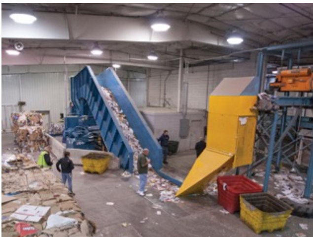
Figure 16: Recycle materials loaded onto below ground conveyor belt into hopper above baling chamber
