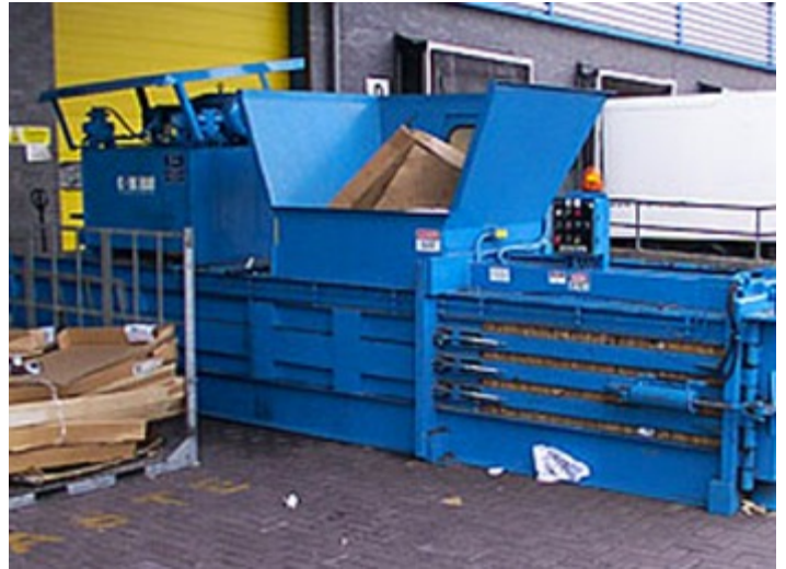
Figure 14: Recycle materials loaded into hopper above baling
