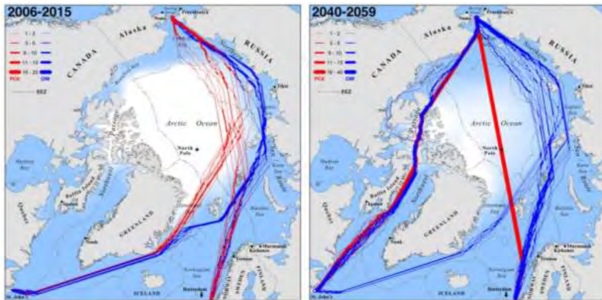
Figure 4. Current Ice Coverage (left) and Predicted Change in Ice Pack with Predicted New Routes (right)
