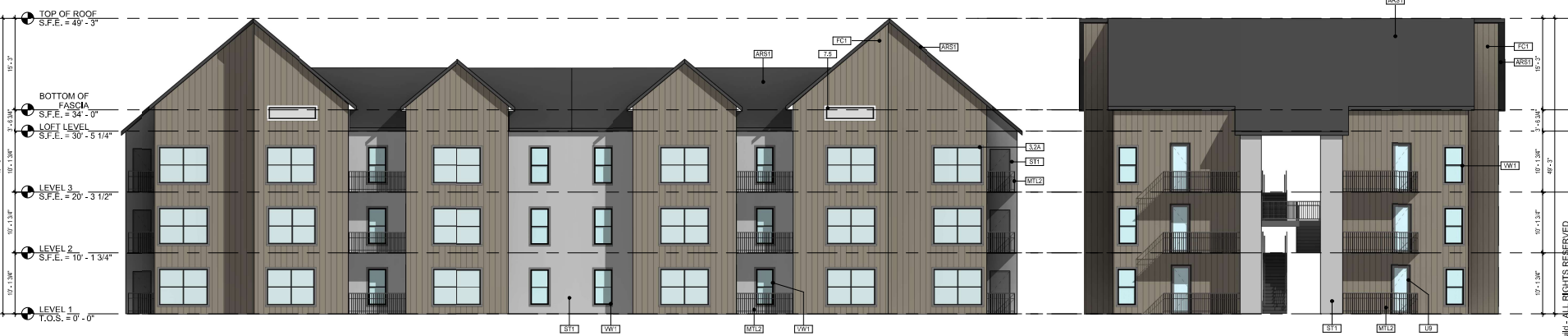
2 SOUTH ELEVATION - BUILDING 300 1/8" = 1'-0"
