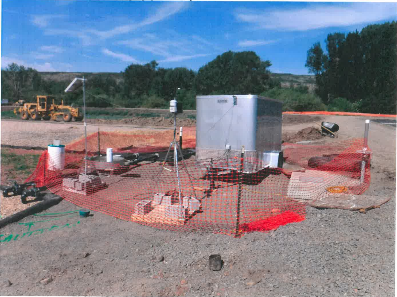
Figure 1: Example Seepage Testing Equipment Setup
