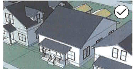
1. As illustrated above, new dormer(s) have been added to a rear-facing roof plane to be less visible from the street and sidewalk. A rear dormer or dormers may provide an opportunity for a small building addition as illustrated on page 66.
