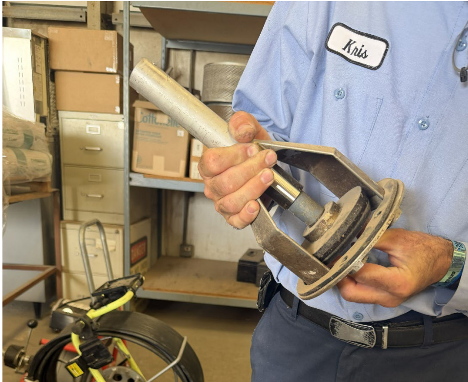
Figure 11. The solids excluding valve, which is controlled by pressure/head loss differential, was shown in the open and closed position.
