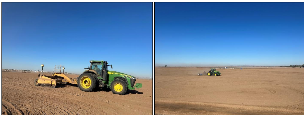
Tractor pulling a GPS levelling machine to dead-level a produce field (left); tractor pulling a laser-levelling machine, with laser station visible as a small blue tower in the right-center of the frame (right).
