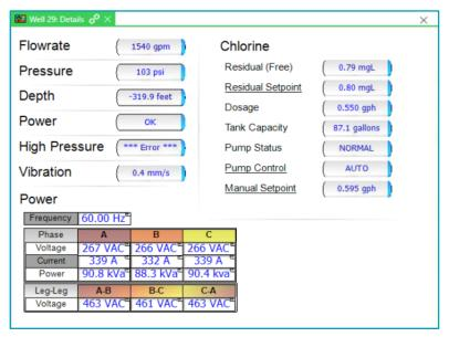
Well 29 Real-Time Well Sounding – Staff installed a sonar-based, automatic, realtime well sounder that is now logging groundwater levels into SCADA. The image below is the display interface that is in the field. (note: this image was taken prior to calibration and is not the actual measurement)
