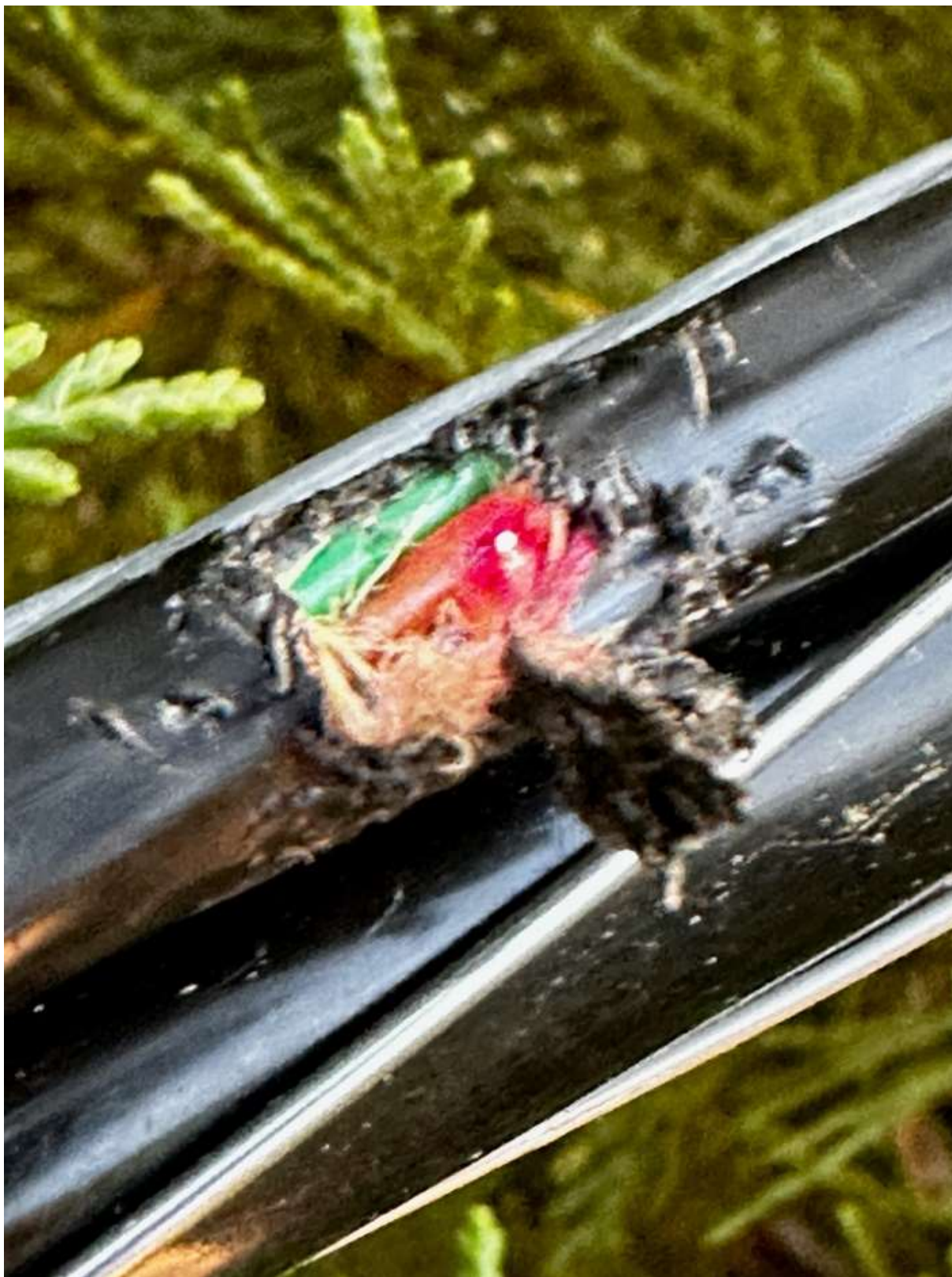
A single squirrel chew in a 30+ mile fiber route that had to be located and repaired. This incident occurred twice in the month of April and both times required several hours of repair time.
