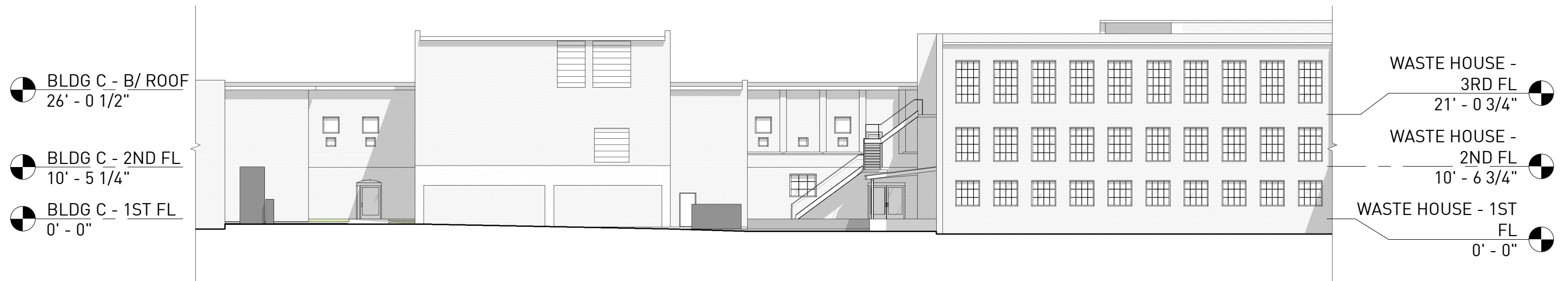
1 EXISTING NORTH ELEVATION SD-3.1 1" = 20'-0"
