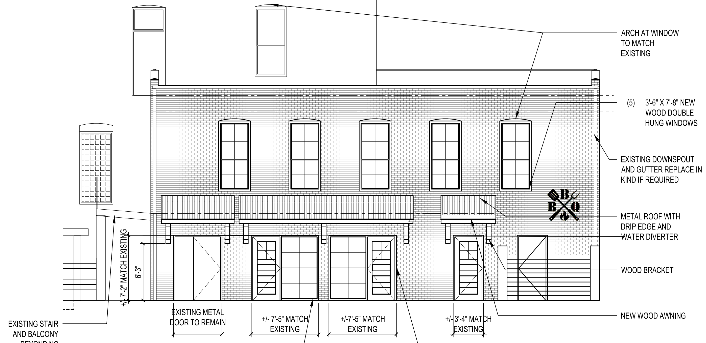
2 EXISTING ELEVATION WITH NEW FENESTRATION 3/16" = 1'-0"
