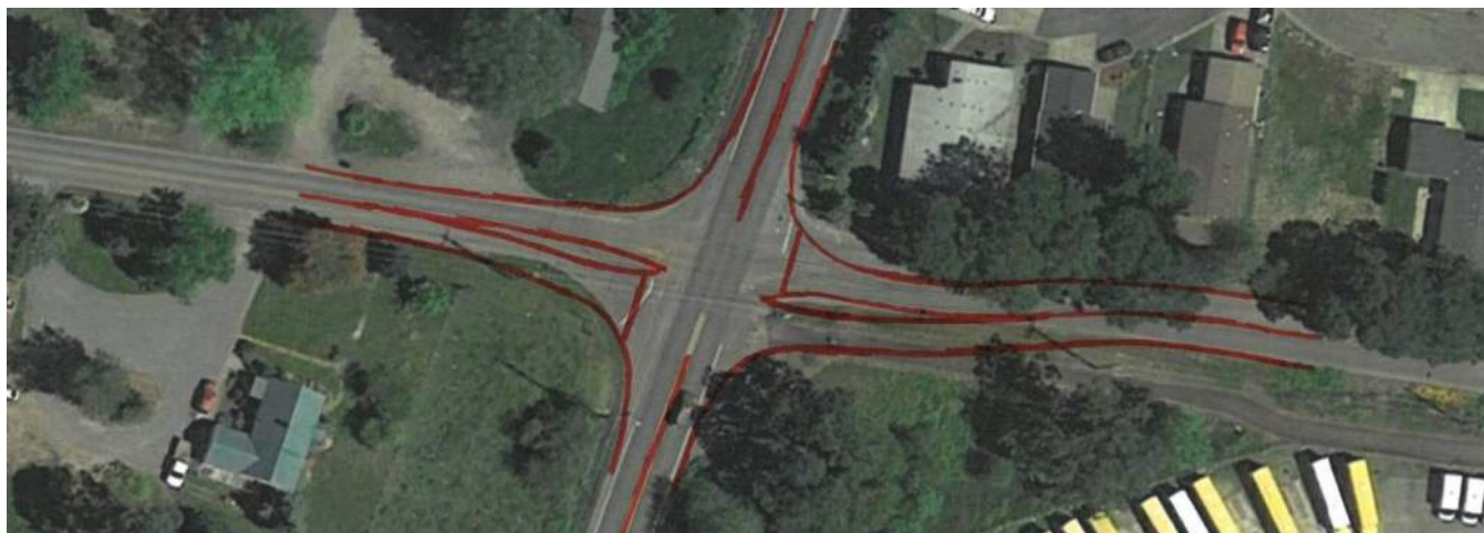
Illustration of concept to align the eastbound and westbound approaches to the intersection
