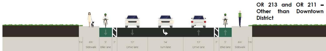
Arterial with Buffered Bike Lanes and Center Turn Lane (68-foot ROW, 52-foot Paved Width)
