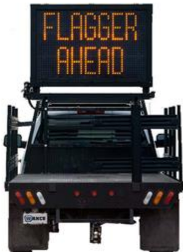
Wanco Truck Mount Message Board Sign, Arrow Board, and Full Graphic Display WVMBM, for Flat bed or Pickup Truck
