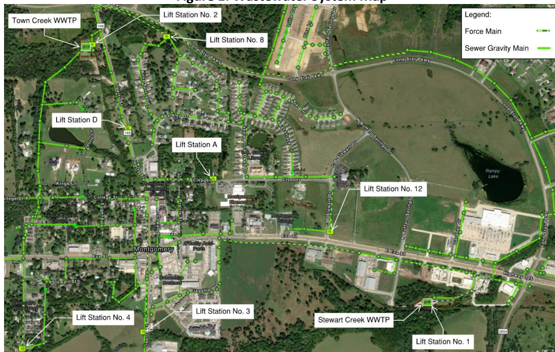
Figure 1: Wastewater System Map
