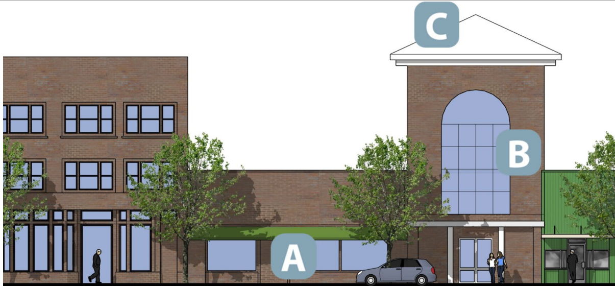
Figure Notes: A = Building Base | B = Building Body | C = Building Cap
