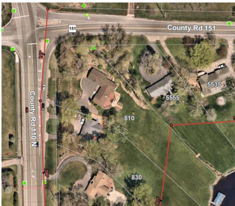
Figure 5. Storm (green) and sanitary (red) sewer at CR 110 & CR 151
