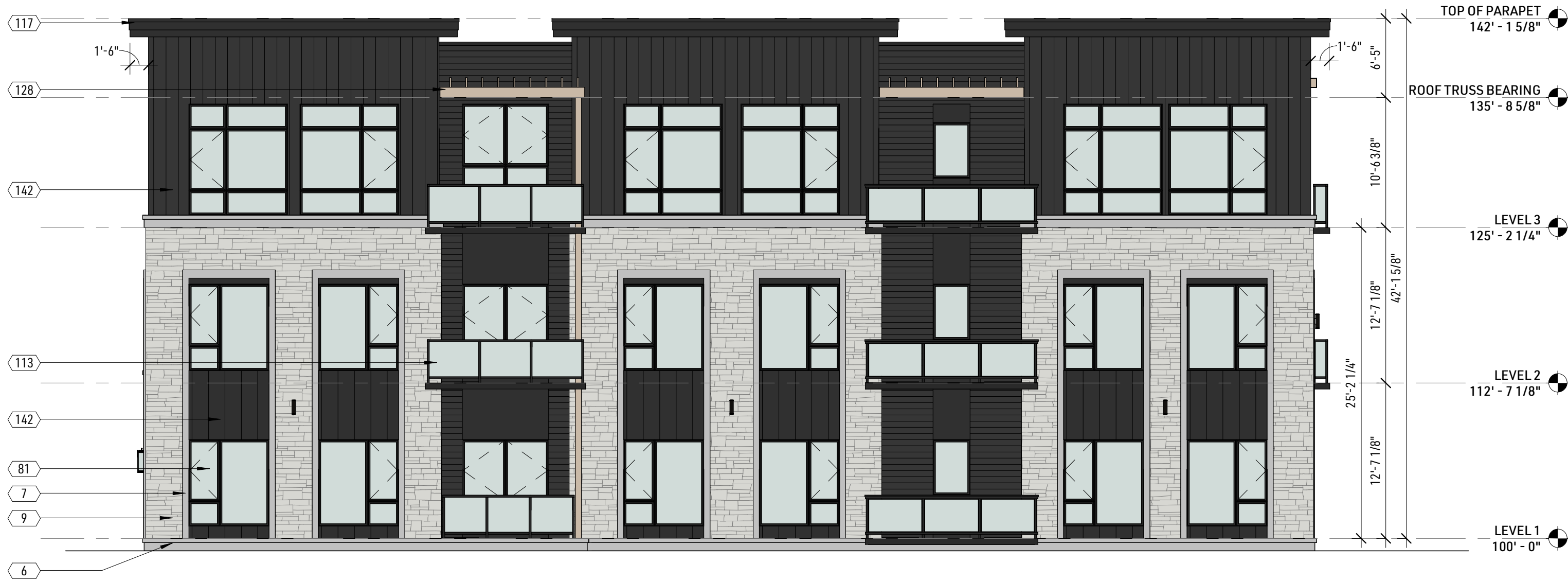
4 WEST EXTERIOR ELEVATION 1/8" = 1'-0"
