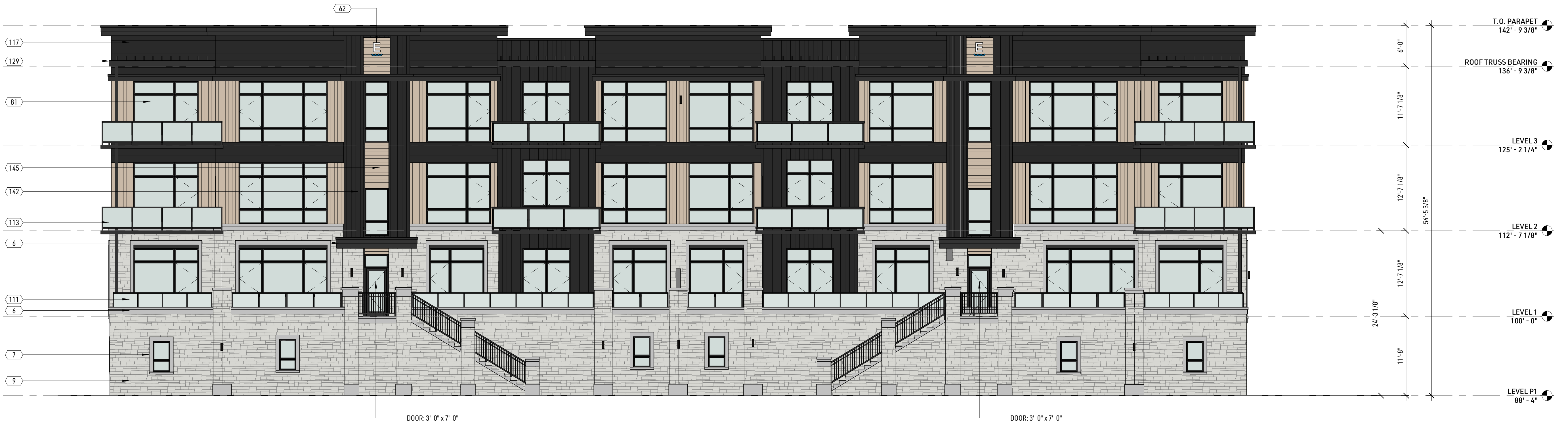
3 SOUTH EXTERIOR ELEVATION 1/8" = 1'-0"
