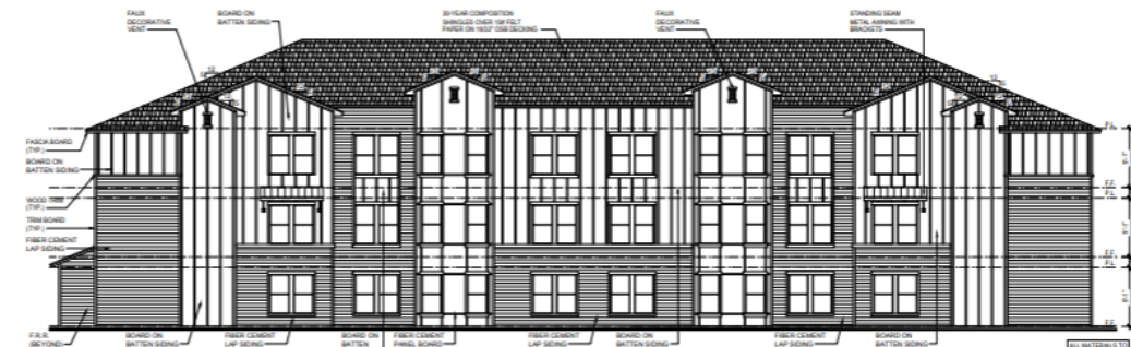
04 BUILDING 'B' - REAR ELEVATION SCALE: 1/8" = 1'-0" 1 RECD @ BLDG #2
