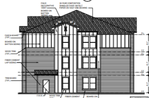
02 BUILDING 'A' - RIGHT ELEVATION SCALE: 1/8" = 1'-0"
