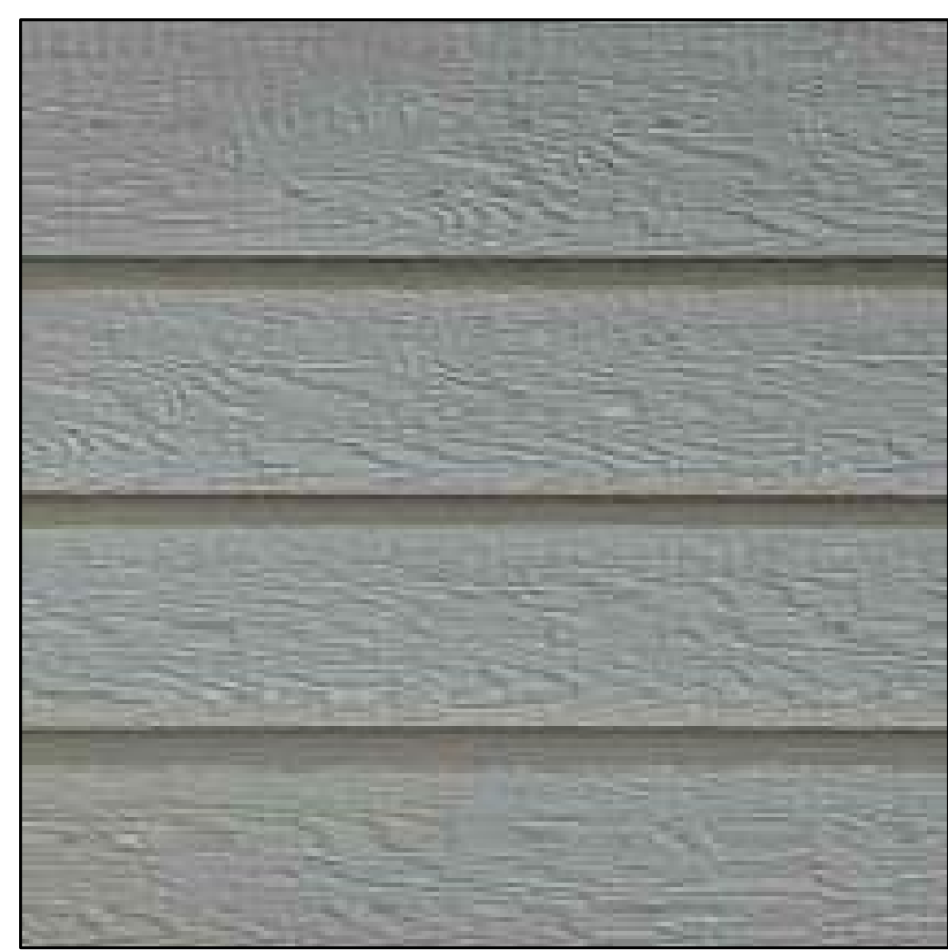
LAP SIDING EXAMPLE MATERIAL EXAMPLE ONLY NOT FOR COLOR
