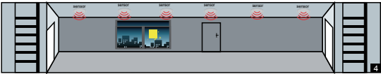
4. After stand-by period, the lamps switch off if no movement is detected in the detection zone.
