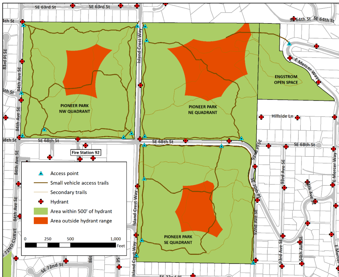
Figure 3: Fire occurrence resources, including small vehicle access, entry points, hydrant locations and secondary trails (see Appendix for larger version)
