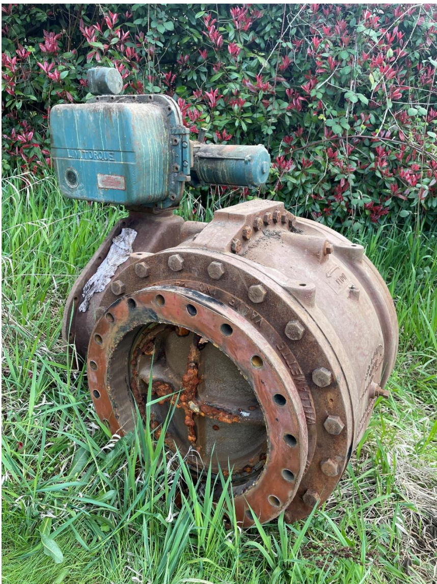
24-in ball valve that stuck closed
