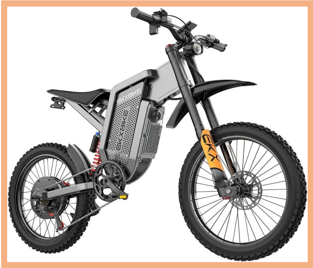
EK X21 Off Road E-Bike 3,000W motor; top speed of 45mph.
