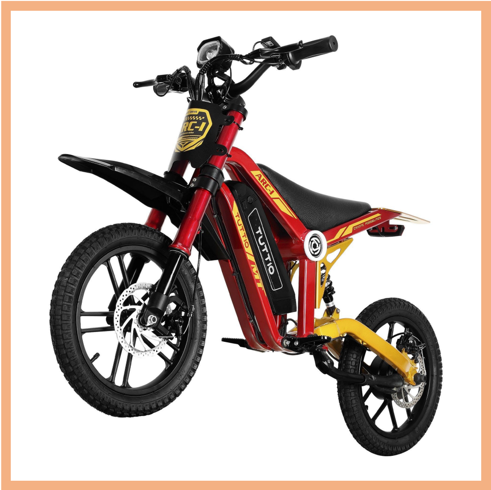
TUTTIO ARC-I Kids Electric Dirt Bike 750W motor; top speed of 22mph; no pedals.
