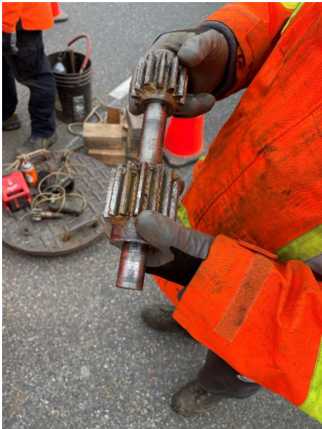
Shear pin broke - top shaft gear came loose (by design to protect gears from damage)
