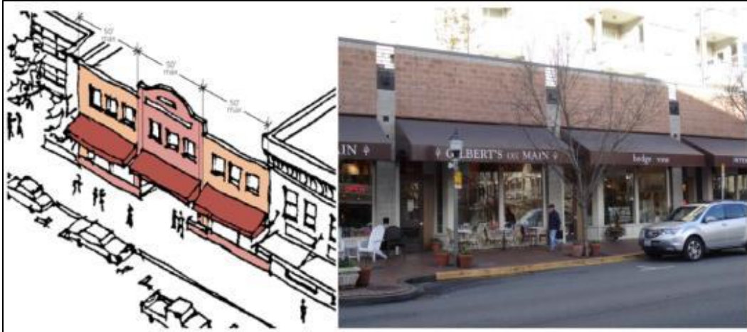
FIGURE 13 — MINOR FACADE MODULATION EXAMPLES
