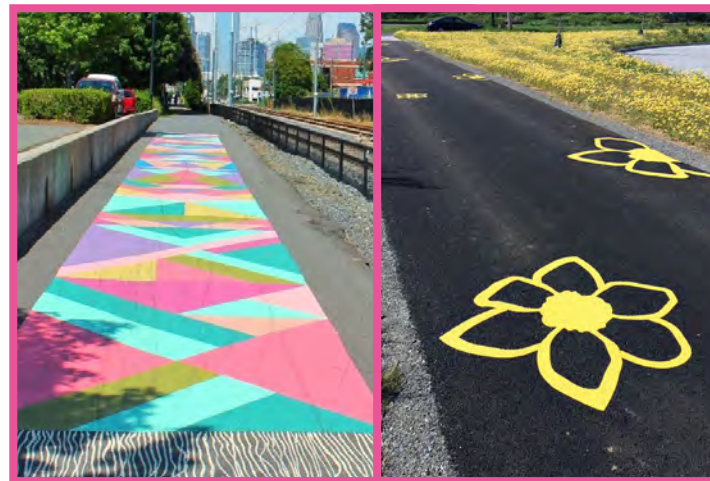
colored surface pavement treatment examples
