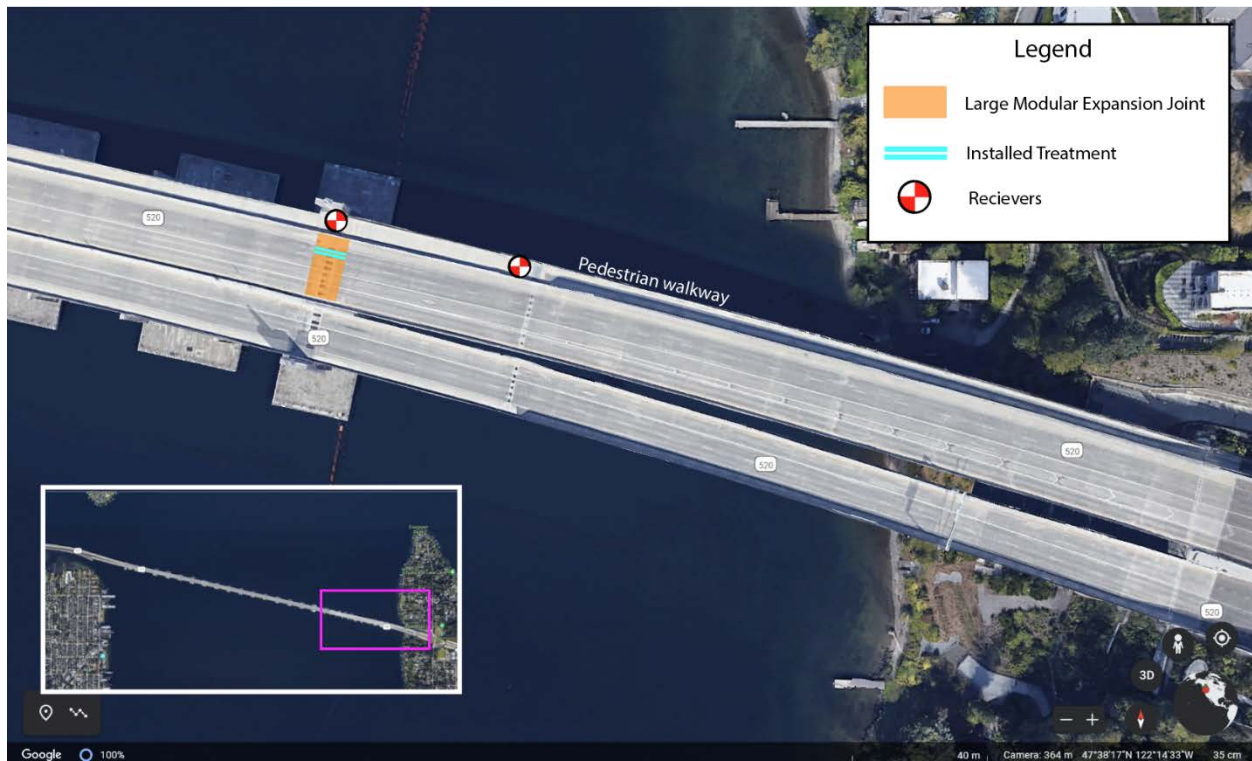
Figure 4-5. Map showing expansion joint and sound measurement locations.
