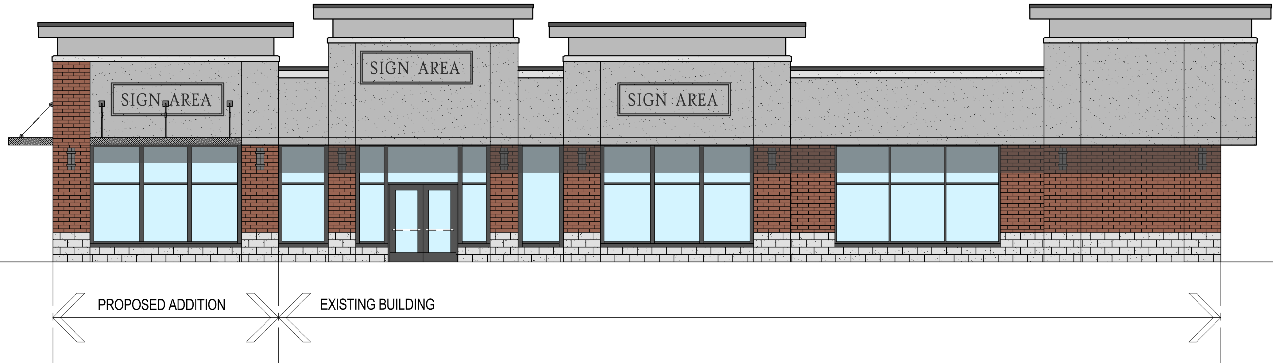
3 PROPOSED NORTH ELEVATION A202 SCALE: 1/8" = 1'-0"
