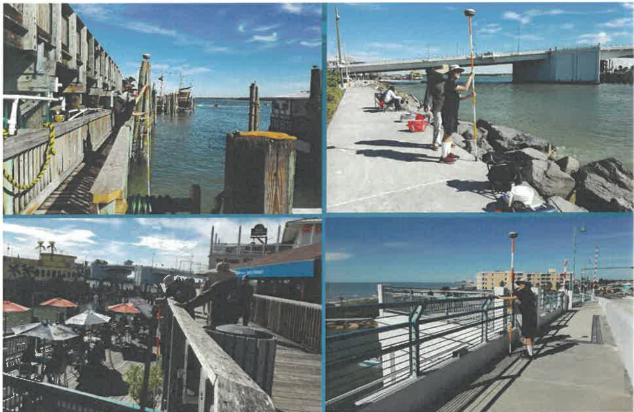
Figure 17. Survey of land boundary and the bridge piling positions using RTK GPS.
