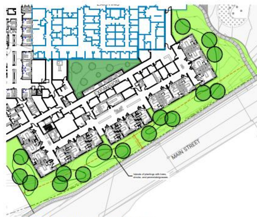
1 Alternate 1: Vault Option for Stormwater: Under building vault with frontage landscape bermed with lawn and trees, and islands of landscape.
