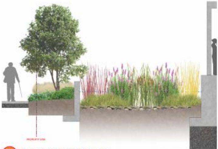
P Preferred Option for Stormwater: Stormwater swale at entry and frontage. Cobble/river rock in base of swale, with irrigated landscape including dogwood shrubs, spirea douglasii, cattail and juncus.
