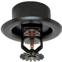
At occupied rooms, the sprinkler heads are intended to be semi-recessed, with projections below ceiling level limited to that necessary for proper flow distribution. The "deep escutcheons" are intended to accommodate the maximum recess allowable for the selected head.
