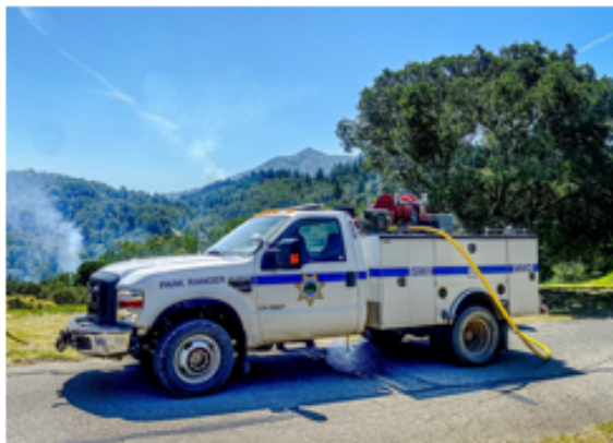
Ranger Type 6 supplying a hose line at a recent burn.
