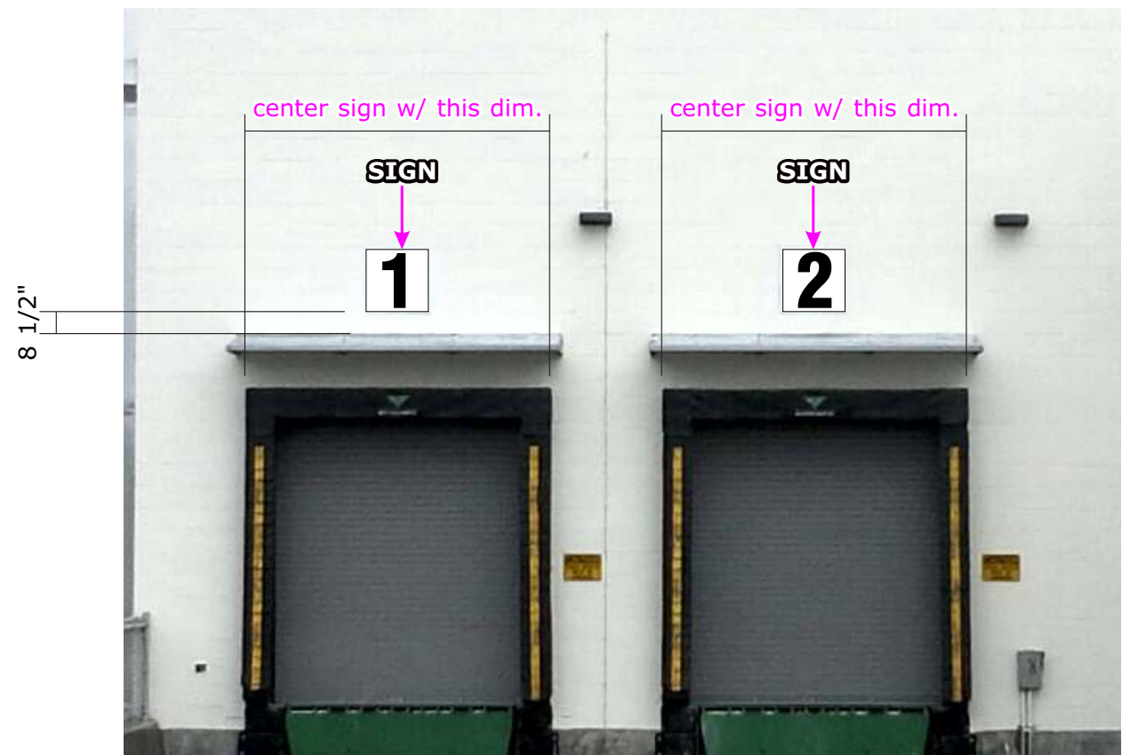
TYPICAL EXTERIOR DOCK SIGNS
