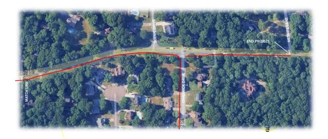
The City has requested TTL's assistance in preparing preliminary designs for the Eastview Drive and Chadwick Lane sidewalk segments including anticipated alignments, opinion of probable costs, evaluation of potential project constraints, and a proposed phasing plan should the City choose to complete the project in multiple stages.
