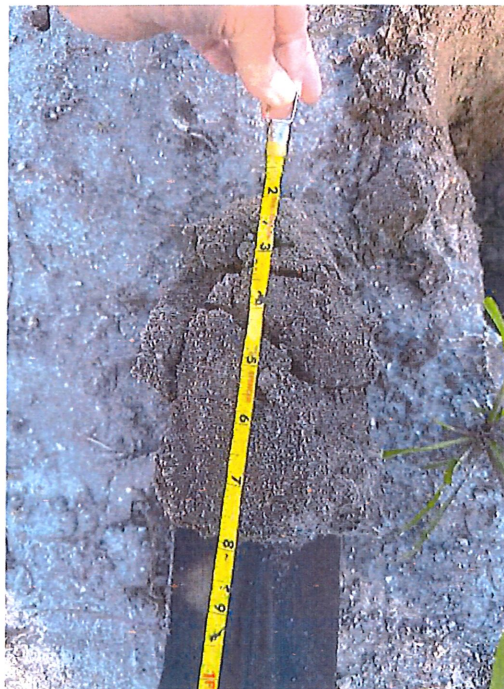
Apparent shell rock fill material t placed in center of lot and around existing trees
