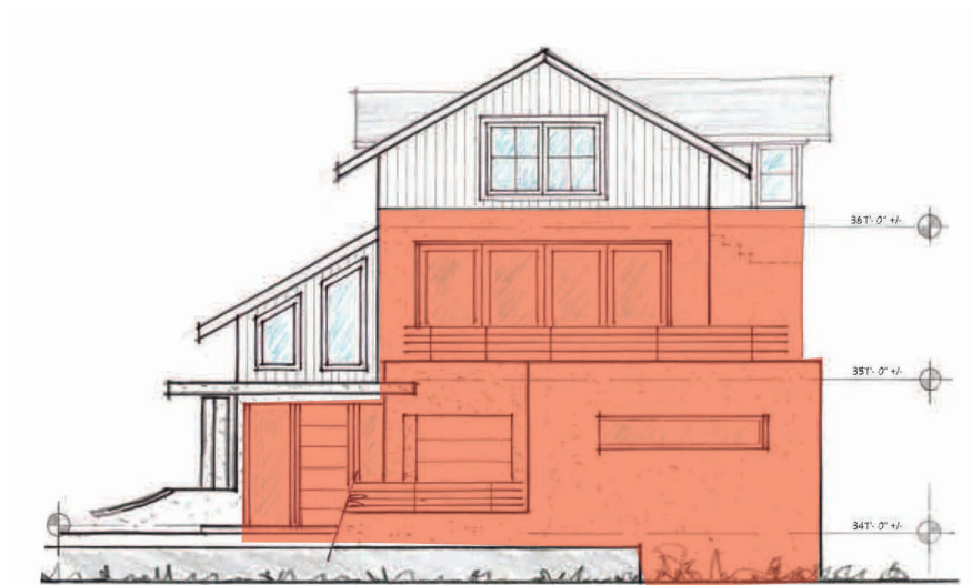
Large amount of stucco would be out of character with this neighborhood and not consistent with Residential Design Guideline 3.8.2
