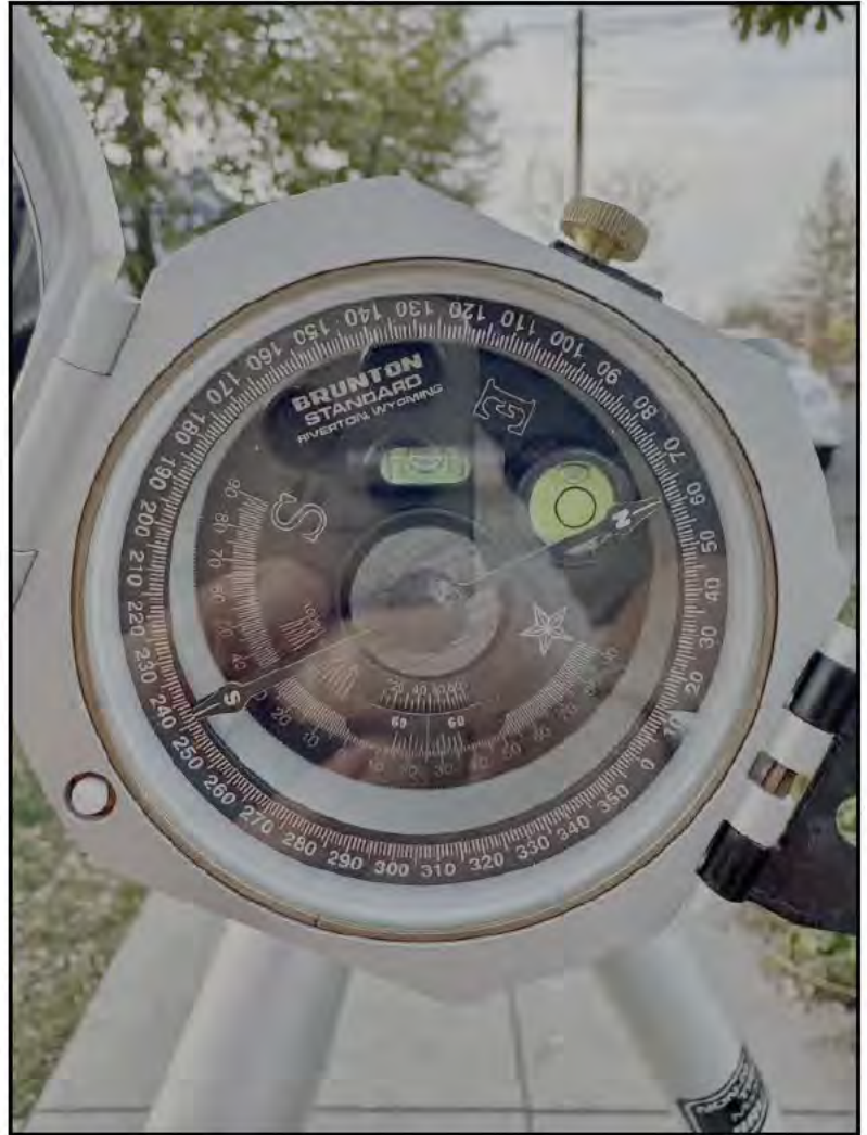
2 Adjust the vernier to determine the inclination of the roof from the transit ( \theta )
