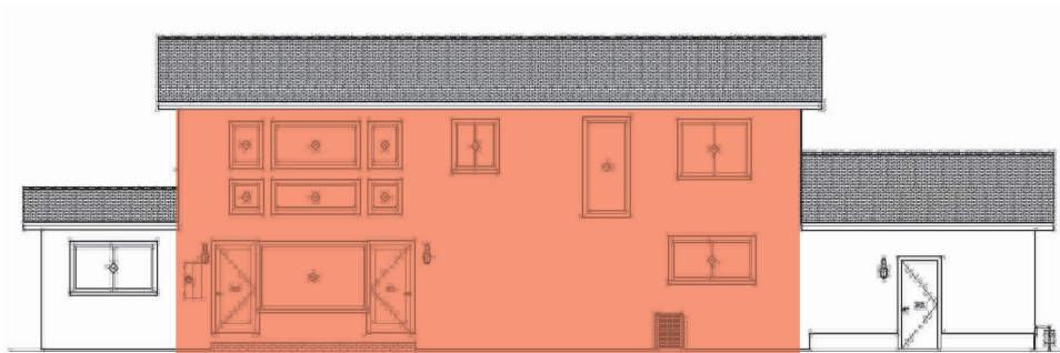
The two story single plane wall would not be consistent with Residential Design Guideline 3.3.3
