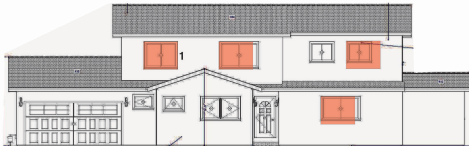
The large variety of window sizes and proportions is chaotic and would not be consistent with Residential Design Guidelines 3.7.1 and 3.7.2
