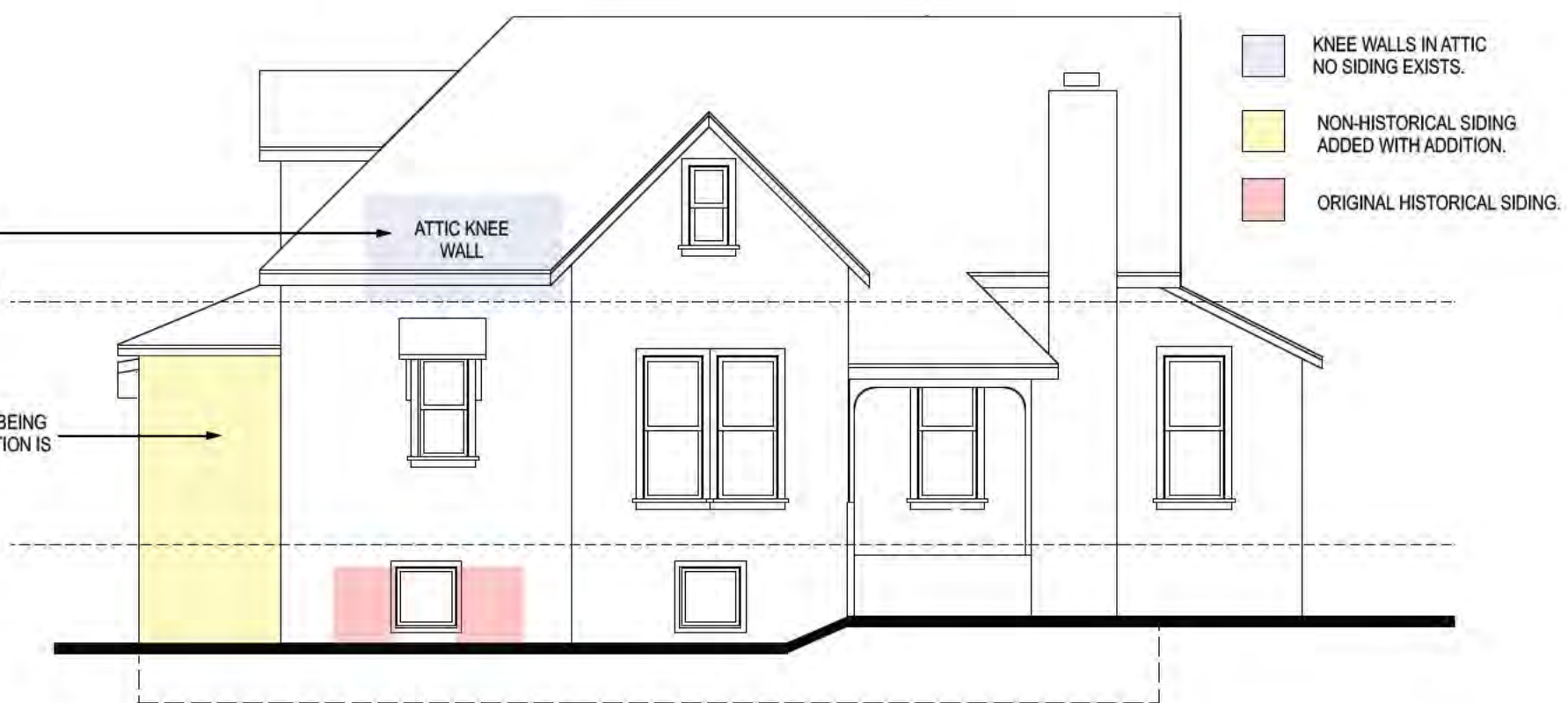
896 SF OF EXTERIOR WALL SIDING. 113 SF OF EXTERIOR WALL SIDING REMOVED. (13%) FACING A PUBLIC STREET. EXISTING LEFT SIDE ELEVATION (NORTHWEST) 1/8" = 1'-0"
