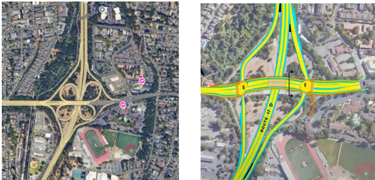
Exhibit 3.2: Modification of the SR 17/SR 9 Interchange from the Current Cloverleaf Configuration (left image 32 ) to a Partial Diamond Configuration (right image 33 )
