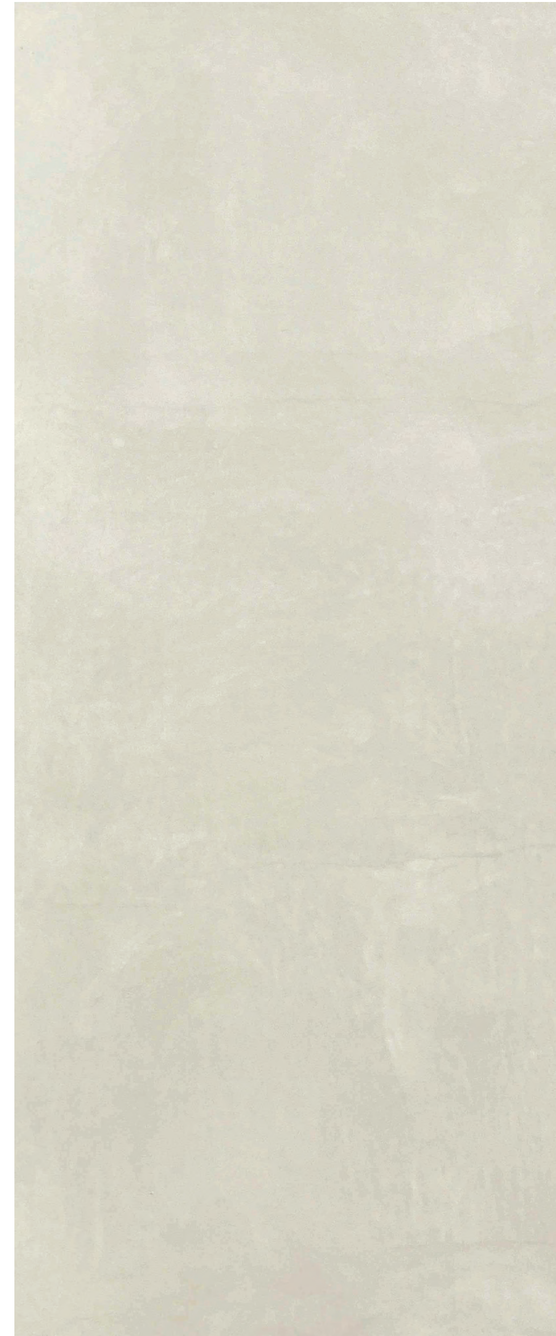
STU-1 STUCCO SYSTEM MFR: RICK MARS EXTERIOR CLADDING LIGHT CREAM PROPRIETARY 5 COAT VENETIAN PLASTER CUSTOM FINISH PER OWNER REQUIREMENTS
