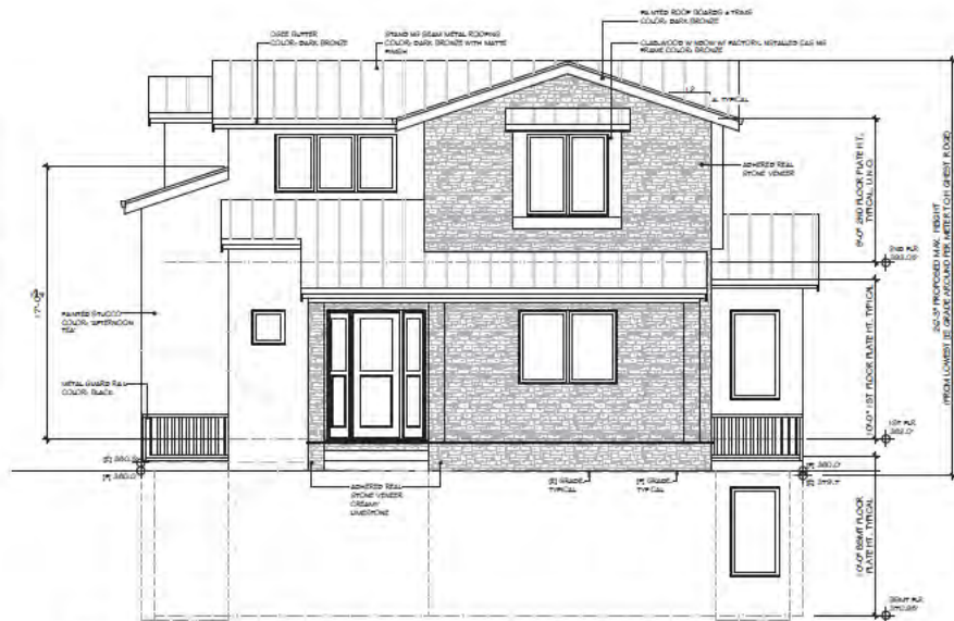
FRONT (SOUTHWEST) ELEVATION 1/4" = 1'-0"
