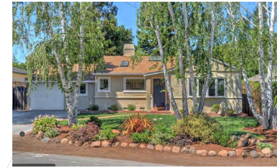
481 SAN LUIS AVENUE HOUSE STYLE: TRANSITIONAL NUMBER OF STORIES: 1 EXT. MATERIALS: STUCCO ROOF STYLE: HIP/GABLE ROOF MATERIALS: COMP SHINGLE
