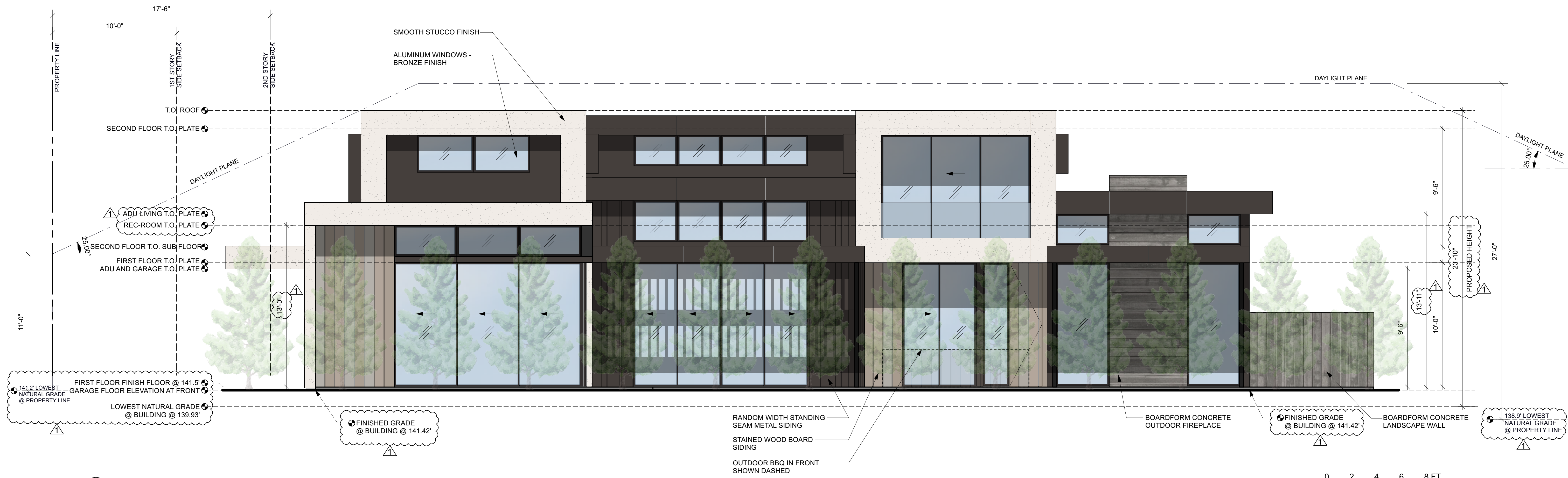
2 EAST ELEVATION - REAR Scale: 1/4" = 1'-0"
