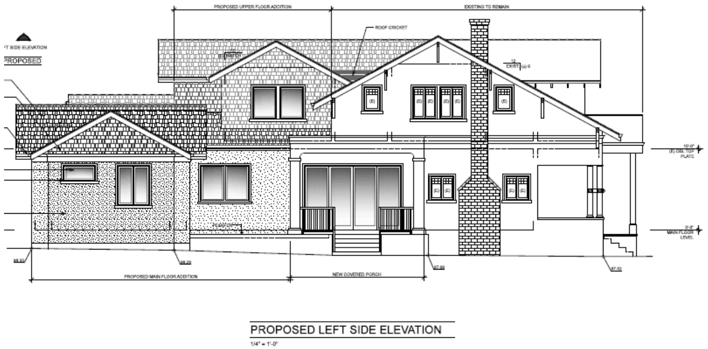
Figure 5 -B 236 Eleanor Avenue- Rehabilitation Plan View: Left (South) Facade showing the proposed connection of the new wing. The historic house and front roof structure are shown to remain at a height above the proposed addition. The roof structure is intersected with the new roof structure to create a cross gable in the second story. Source: Chapman Design Associates, Jacobsen/Parmacek Residence Sheet A4.0
