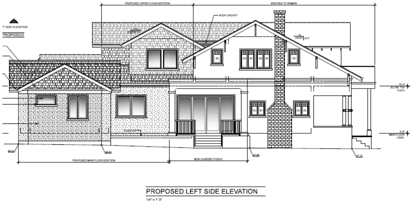
Figure 5 -B 236 Eleanor Avenue- Rehabilitation Plan View: Left (South) Façade showing the proposed connection of the new wing. The historic house and front roof structure are shown to remain at a height above the proposed addition. The roof structure is intersected with the new roof structure to create a cross gable in the second story. The plan results in the loss of historic siding materials. Source: Chapman Design Associates, Jacobsen/Parmacek Residence Sheet A4.0
