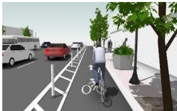
Buffered Bike Lane with Vertical Element (Class IV)
