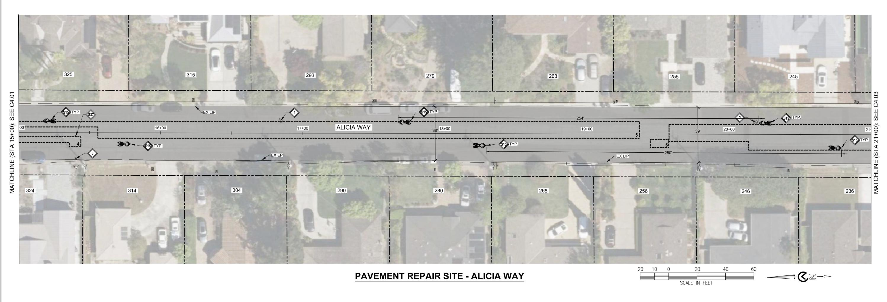
LOWER & RESTORE TO GRADE SEWER MANHOLE (TEMPORARY FALSE BOTTOM TO BE INSTALLED PRIOR TO ANY MANHOLE WORK, & REMOVED AFTER)
