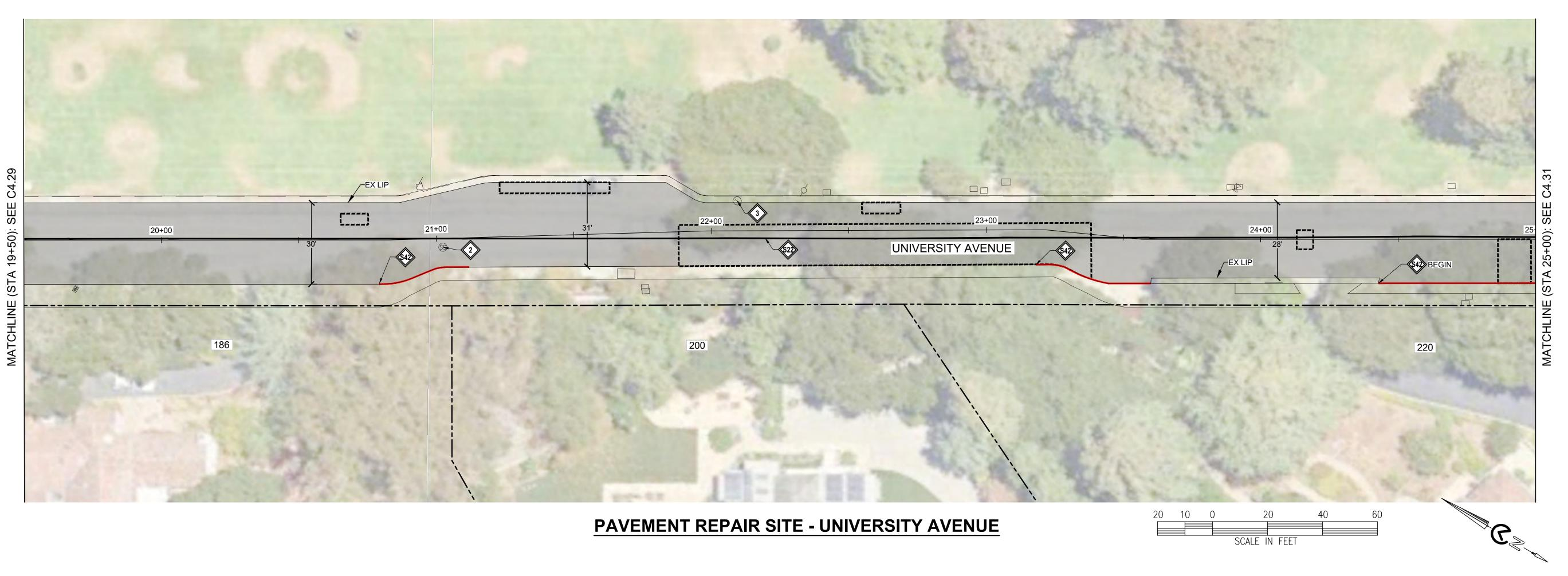
LOWER & RESTORE TO GRADE SEWER MANHOLE (TEMPORARY FALSE BOTTOM TO BE INSTALLED PRIOR TO ANY MANHOLE WORK, & REMOVED AFTER)
