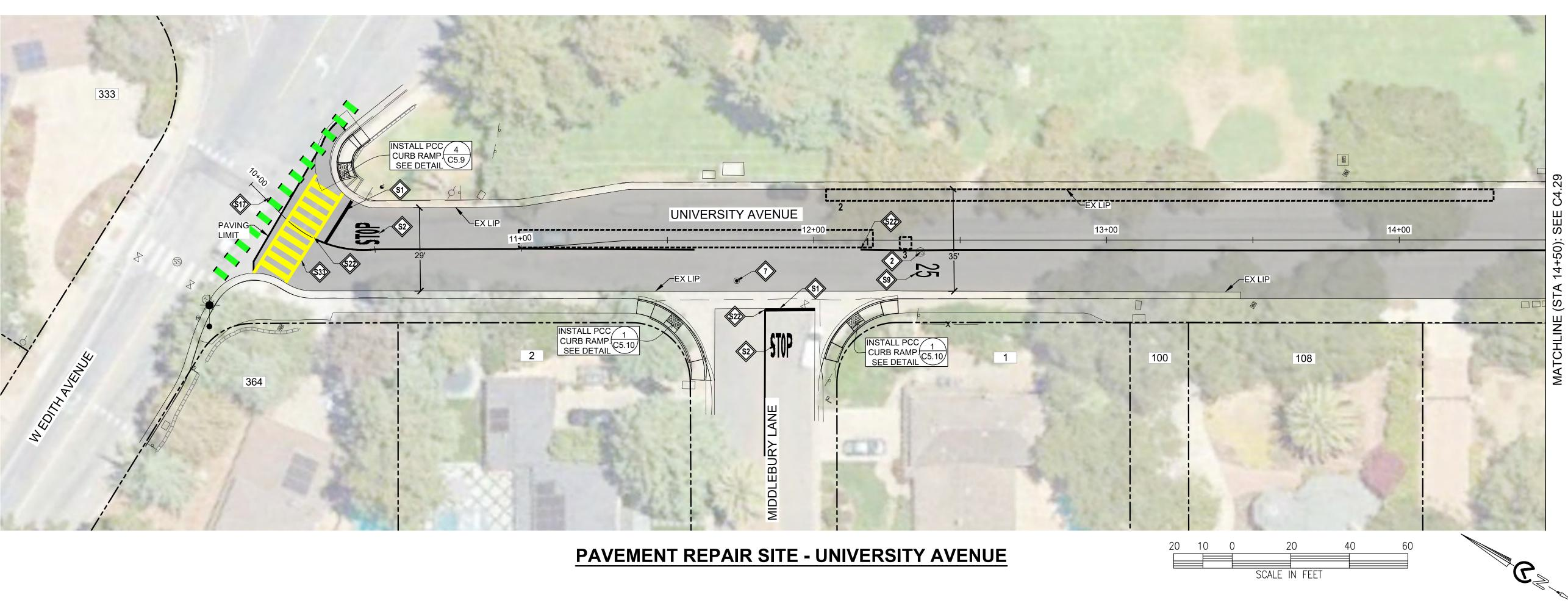
LOWER & RESTORE TO GRADE SEWER MANHOLE (TEMPORARY FALSE BOTTOM TO BE INSTALLED PRIOR TO ANY MANHOLE WORK, & REMOVED AFTER)
