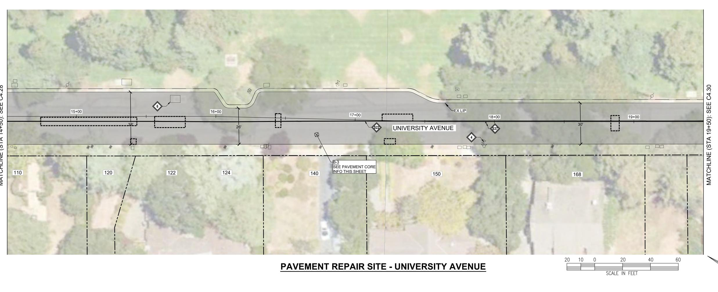
LOWER & RESTORE TO GRADE SEWER MANHOLE (TEMPORARY FALSE BOTTOM TO BE INSTALLED PRIOR TO ANY MANHOLE WORK, & REMOVED AFTER)
